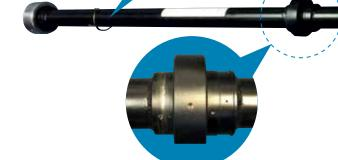
It is important to ensure that the o-ring supplied with the manifold is inserted into the end cap before it is tightened up. The 90-115mm 'C' Spanner (Part No. 35017403, not supplied) is used to assemble the manifold sections and also tighten the end cap.
