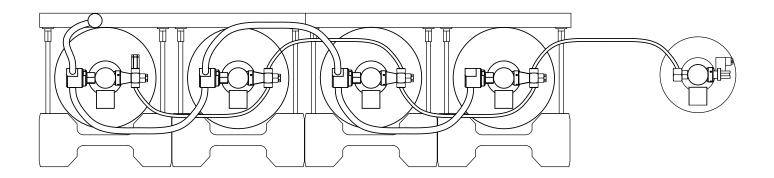
The plug (blind cap and dowty seal) on the hose connector will need to be removed and discarded to allow connection of the discharge hose/hoses.
