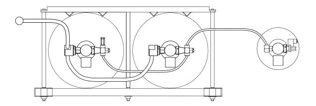
The plug (blind cap and dowty seal) on the hose connector may need to be moved to the other port depending upon the final system arrangement used. Please ensure that the plug is securely tightened on the hose connector during installation, even if it hasn't been moved to another port.
