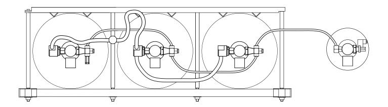
The plug (blind cap and dowty seal) on the hose connector may need to be moved to the other port depending upon the final system arrangement used. Please ensure that the plug is securely tightened on the hose connector during installation, even if it hasn't been moved to another port.
