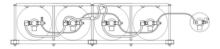
The plug (blind cap and dowty seal) on the hose connector may need to be moved to the other port depending upon the final system arrangement used. Please ensure that the plug is securely tightened on the hose connector during installation, even if it hasn't been moved to another port.
