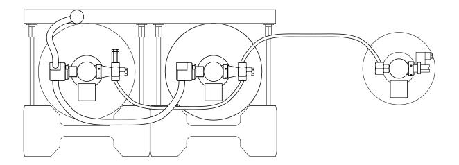
The plug (blind cap and dowty seal) on the hose connector may need to be moved to the other port depending upon the final system arrangement used. Please ensure that the plug is securely tightened on the hose connector during installation, even if it hasn't been moved to another port.
