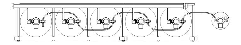
For systems with more than four 140L containers a manifold must be used. Please note that the manifold supports are not shown for clarity.
