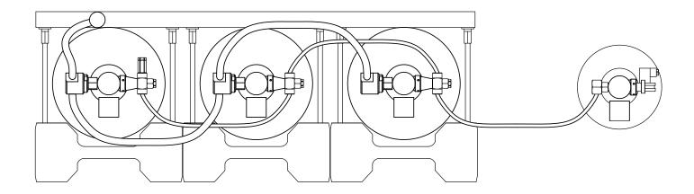
The plug (blind cap and dowty seal) on the hose connector may need to be moved to the other port depending upon the final system arrangement used. Please ensure that the plug is securely tightened on the hose connector during installation, even if it hasn't been moved to another port.
