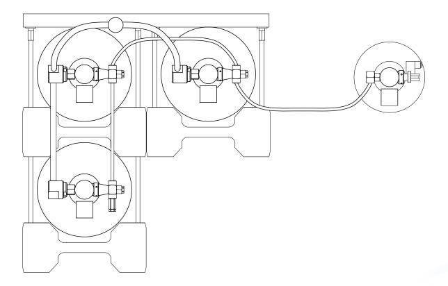
The plug (blind cap and dowty seal) on the hose connector will need to be removed and discarded to allow connection of the discharge hose/hoses.
