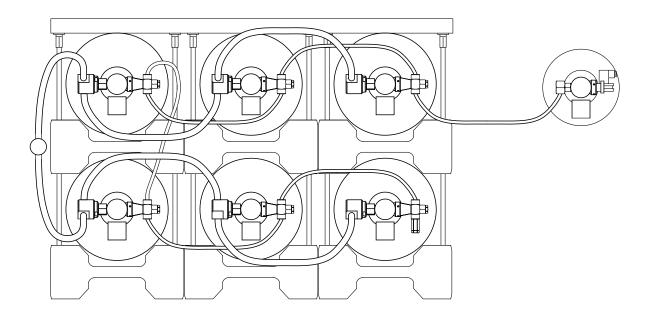
The plug (blind cap and dowty seal) on the hose connector will need to be removed and discarded to allow connection of the discharge hose/hoses.
