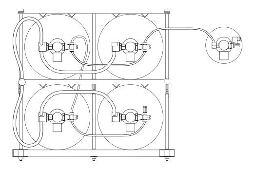
The plug (blind cap and dowty seal) on the hose connector may need to be moved to the other port depending upon the final system arrangement used. Please ensure that the plug is securely tightened on the hose connector during installation, even if it hasn't been moved to another port.
