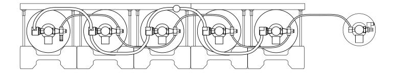
The plug (blind cap and dowty seal) on the hose connector will need to be removed and discarded to allow connection of the discharge hose/hoses.
