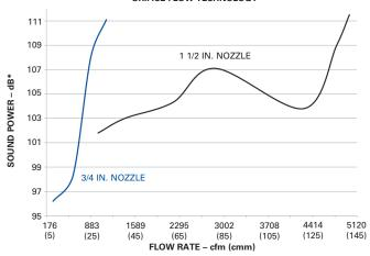
\*Sound power in dB re 1 picoWatt vs. cubic feet (meters) per minute (cfm (cmm)) flow rate
