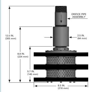
FIGURE 1 1 1/2 IN. NOZZLE DIMENSIONS
