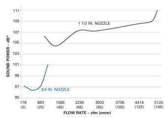
\*Sound power in dB vs. cubic feet (meters) per minute (cfm (cmm)) flow rate
