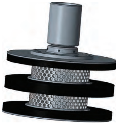
Figure 8: Acoustic Nozzle Exterior View
